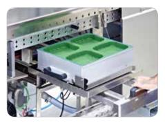
**Change in format** A fast format-changing system in all the thermoformers utilising unique folding moulds, extraction rails, etc. depending on model.
